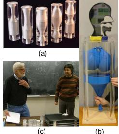
of interest in seeing and hearing real models of the vowels Figure 2. (a) Arai's models of human with an excitation source. They were mainly interested in vocal tract as educational tools. (b) A the different shapes for the vowels, and the capability to lung model. (c) Arai's models used in a simulate a variety of other shapes (Stevens, 2004). class by Stevens.
