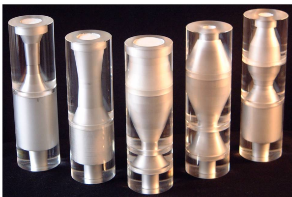
Figure 1: The earliest version of Arai's "cylinder-type" models. The internal vocal-tract shape is sculpted from a transparent acrylic bar [1,2]. The vowels are /i/, /e/, /a/, /o/, and /u/ from left to right (the glottis is at the bottom, the lip is at the top).
