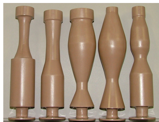
Figure 2: The second generation of Arai's "cylinder-type" models. The internal shapes are exactly the same as the earlier models in Fig. 1, but the thickness of the wall of these models is constant (2.5 mm). The models are made of a material called "chemical wood" in this figure. The vowels are /i/, /e/, /a/, /o/, and /u/ from left to right (the glottis end is the bottom, the lip end is the top).
