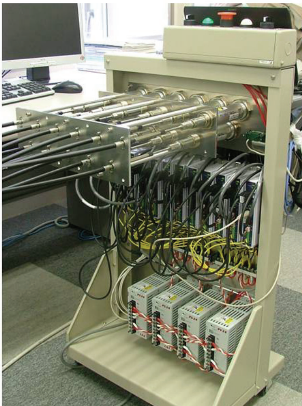
Figure 3: Computer-controlled Umeda & Teranishi model. Each one of the eleven strips is hard-wired to each actuator, and the position of each time frame is controlled by a programmable logic controller.
