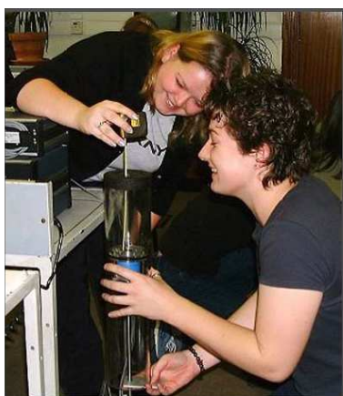
Figure 3. For more than 40 years, acoustics teaching has included hands-on lab practicals for every participant, with specially-developed apparatus. Here Speech Sciences students are introduced to the essential nature of formants by measuring the characteristics of an acoustic resonator. After confirming that the same laws govern mechanical, acoustic and electrical resonators, students are led to understand the use of electrical resonators in signal analysis.
