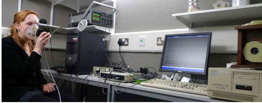
Figure 2. Inside one of the recording rooms. The experimenter is using a Rothenberg mask to gather airflow data. On the bench are a portable Laryngograph, calibration equipment for the airflow unit, and a PC adapted for multi-channel acquisition.
