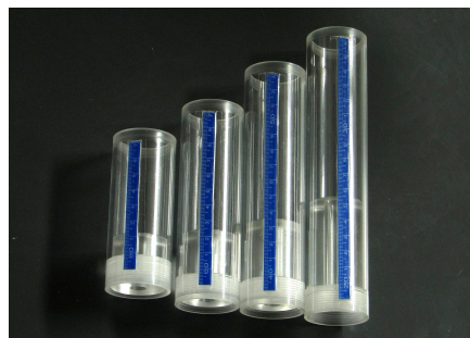
Figure 2: The four versions of the S3T model with the four different combinations of outer and inner cylinder lengths used in this study.
