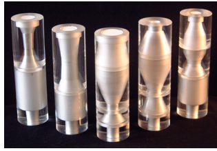
Figure 2: Cylinder-type models of the human vocal tract for producing vowels. The vowels are Japanese /i/, /e/, /a/, /o/, and /u/ from left to right (the glottis end is the bottom, the lip end is the top). The material is acrylic resin. (See more details in [1,2].)
