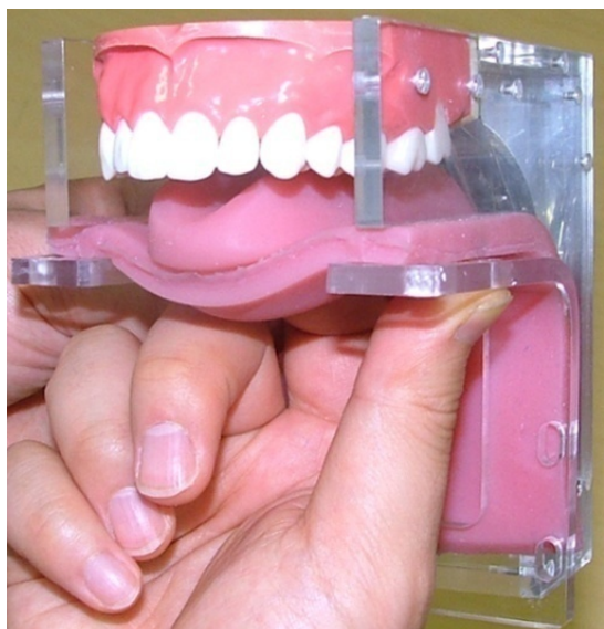
Fig. 1. Physical model of the human vocal tract with a flexible tongue.
